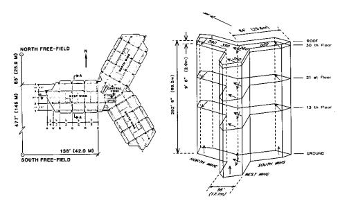
Figure 3. Plan layout and three-dimensional schematic and instrumentation scheme of Pacific Park Plaza (PPP), Emeryville, CA.
