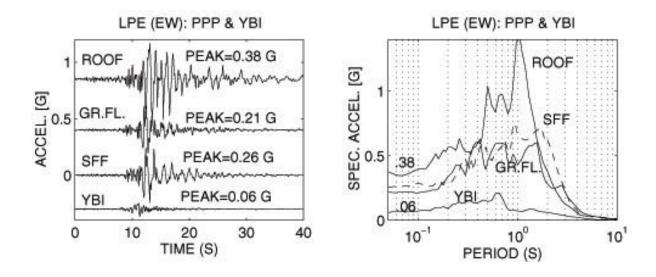
Figure 5. Recorded (EW components) of accelerations and corresponding response spectra at the free-field, ground floor and roof of Pacific Park Plaza (PPP), and at Yerba Buena Island (YBI), at approximately the same distance as PPP, depict the level of amplification.
