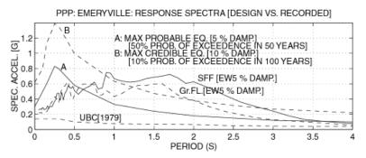
Figure 6. Design response spectra and response spectra of recorded motions at the ground floor and SFF of Pacific Park Plaza. Also shown is the 1979 UBC response spectrum for comparison.
